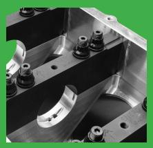
4140 steel billet main caps, ARP main studs with enhanced oiling features.
