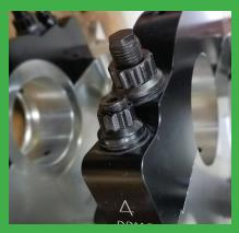
7075 aluminum main caps with  $9/16^{\circ}$  center studs and  $\frac{1}{2}^{\circ}$  splayed outer studs.
