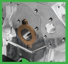
Standard or raised 55mm babbit to 60mm roller cam options, bronze material cam thrust plate included.
