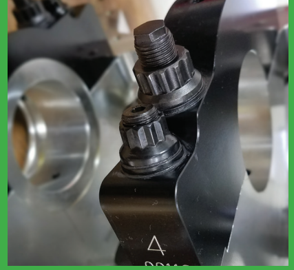
7075 aluminum main caps with 9/16" center studs and 1/2" splayed outer studs.
