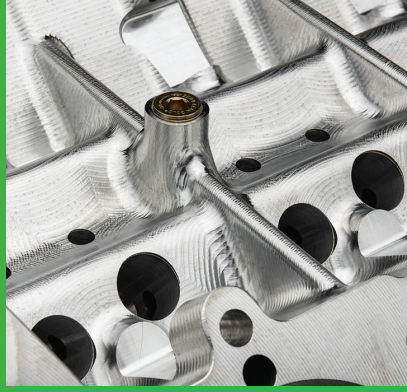
Lifter valley oil galley cross overs with restrictor provisions.
